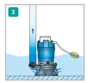
Pump keeps running while the float switch remains on.
