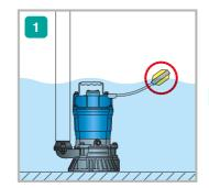
Pump starts operating when the water level rises to a preset level.
